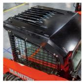
FOPSWW Level 2 For the users that need level 2 FOPS an optional level 2 heavy duty bracket delivers the protection they need. Bracket also protect the front LED work lights.
