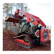
Bucket self-leveling Automatically maintain the bucket position when raising the lift arms.
