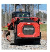
**Counterweight** A rear bumper counterweight improves productivity and protects the rear of the machine from accidental damage. Optional side counterweights can further increase operational capacity.
